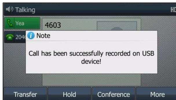
Press **StartREC** to start recording again, the recording will be saved as a new ".wav" file.
