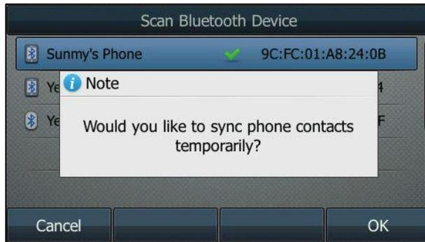
6. (Optional.) Press **OK** to enable the mobile contacts sync feature and the IP phone will sync the mobile contacts temporarily, or press **Cancel** to disable mobile contacts sync feature and the IP phone will not sync the mobile contacts. If you press **Cancel**, you can also manually enable the mobile contacts sync feature on the IP phone. For more information, refer to [Syncing the Mobile Contacts to the IP Phone](#).
