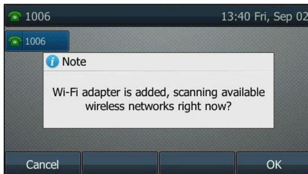
You can press **OK** to activate Wi-Fi mode directly and scan Wi-Fi devices automatically.
