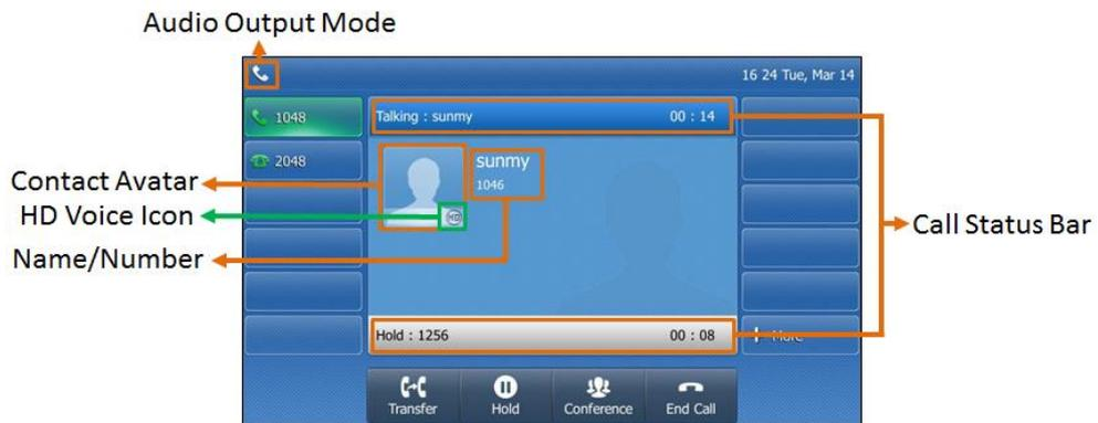
On the SIP-T46S/T46G/T42S/T42G/T41S/T41P/T40G/T40P IP phone you can press up or down navigation keys to switch among calls. When there is an active call and a held call, the Calls screen on SIP-T46S/T46G IP phone is shown as below:
