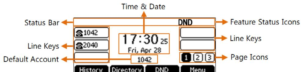
The Idle screen on SIP-T40G/T40P IP phone is shown as below:
