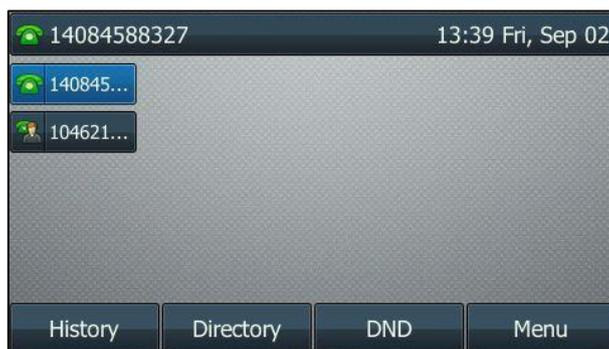
Any IP phone can be used to originate or receive calls on the bridged line. An incoming call to the BLA number can be presented to multiple phones in the group simultaneously, but only one IP phone within the group can answer this call.
