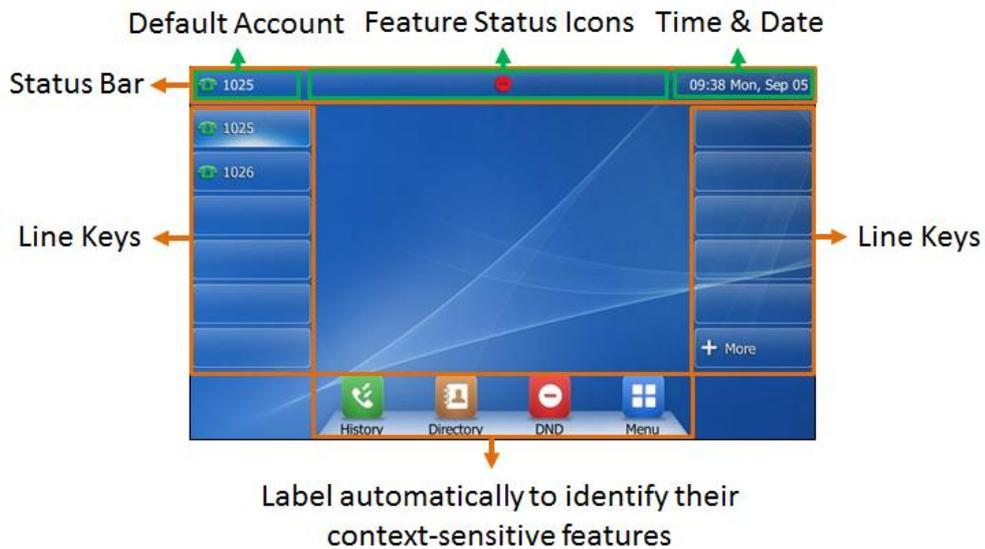
For SIP-T46S/T46G IP phone, the page icons appear only when you assign functionality to line key located in line key 11-27, refer to [DSS Keys](#) for more information. The wallpaper can be customized, refer to [Changing Wallpaper on the Idle Screen](#) for more information. The Idle screen on SIP-T46S/T46G IP phone is shown as below:
